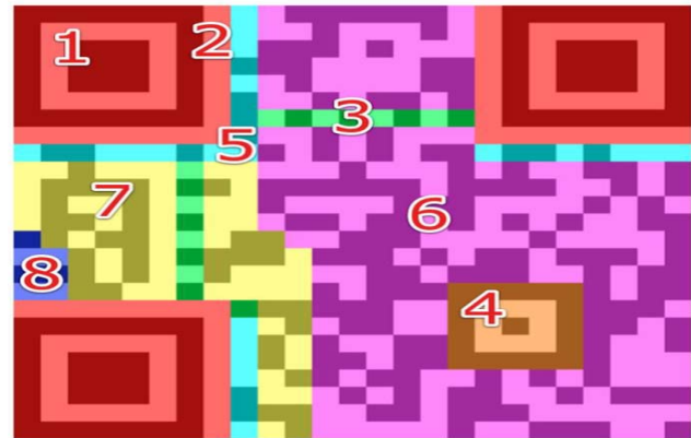
Figure 1: Structure of QR code Version 2
