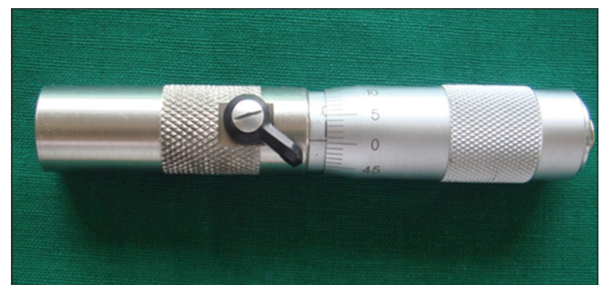
Figure 1: Custom made calibrated depth micrometer
