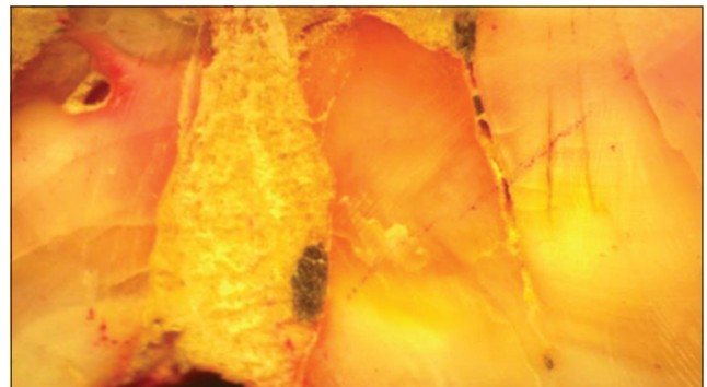
Figure 3: Stereomicroscopic picture showing dye penetration of bone cement
