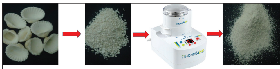
Figure 1: Preparation of seashell reinforced GIC, where seashell biomaterial was collected, initially grounded into a fine homogeneous powder in a mechanical grinder and then transferred to a Smart dentin grinder to obtain a finer mix by micro sieve
