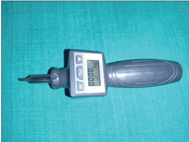
Figure 4: Torque testing screw driver
