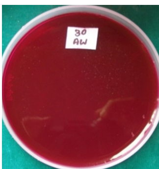
Fig.7: Input bore well water sample tested for presence of E.coli:No contamination seen
