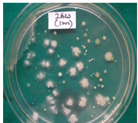
Fig 6: Input borewell water sample: Bacterial contamination seen
