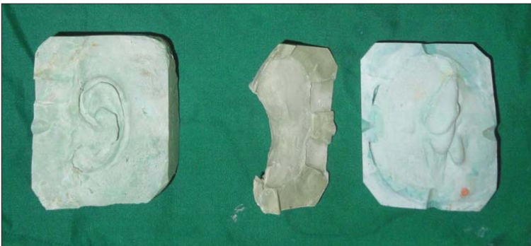
Fig 6: The three part mold after dewaxing
