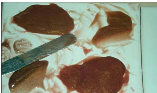
Fig.9: Separation of base shade into various colours
